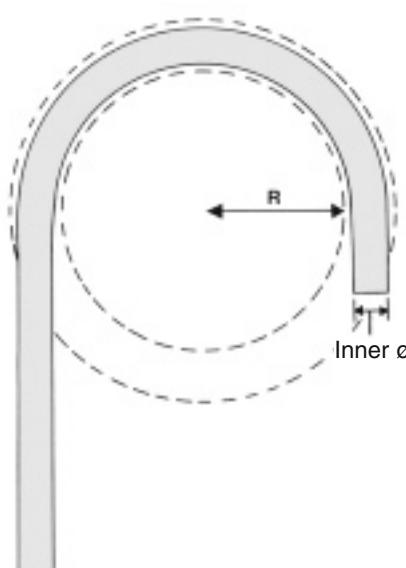
**Bending radius:** „R“ is the radius of the smallest possible circle, to which a hose in service can be bent without damage or shortening its life, by kinking.
